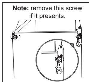
9. Unscrew and remove the bottom hinge pin, turn the bracket over and replace it.
