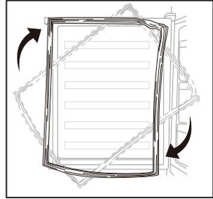
12. Place the door back on. Ensure the door is aligned horizontally and vertically, so that the seals are closed on all sides before finally tightening the top hinge.
