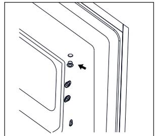
7. Rotate freezer door and place hinge side at left side.
