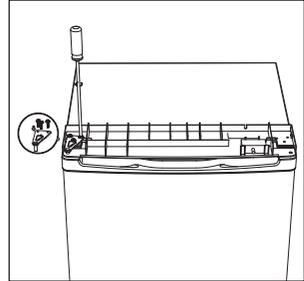
13. Put the top cover and fix it with 2 screws on the back.
