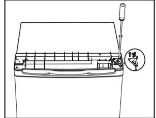
4. Unscrew bottom hinge of freezer door. Then remove the door and place it on a soft pad to avoid scratch.
