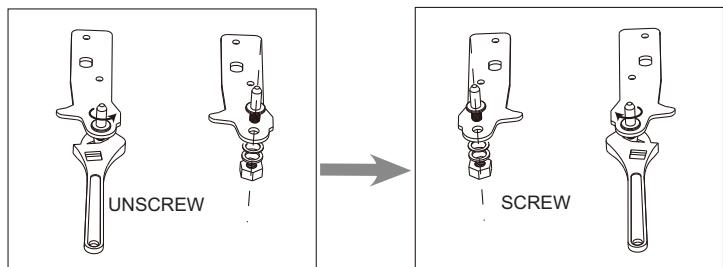
9. Install the hinge at left side and foot base at right side. Then screw two leveling feet with their original parts.
