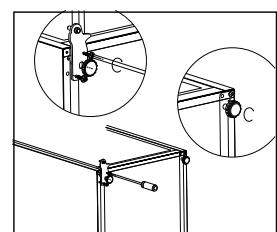
10. Stand up the unit and put the door on the bottom hinge. Make sure the bottom hinge core is inserted in the door hole. Then move the hinge hole cover of bottom door from left side to right side.
