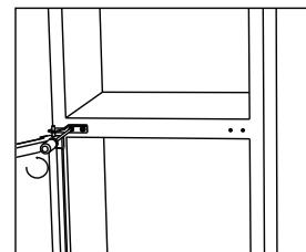
12. Install the upper door with the upper hinge.
