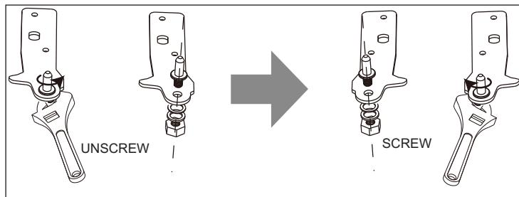
7. Install the hinge at left side and foot base at right side. Then screw two leveling feet with their original parts.
