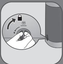
**EN** Set back the draining cap, fully screw it until complete locking and check there is no leakage.
