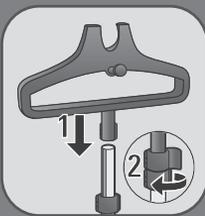
**EN** Unlock the hanger and fully insert it vertically on top of the pole and lock it.
