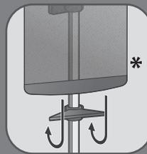
**EN** Unwind the support and insert it in the adjustable hook, by adjusting the tension with the dedicated hook and lock it.
