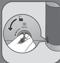
**EN** Place the appliance over a sink & unscrew the «Anti calc» cap by turning it anti clockwise.
