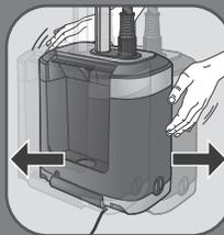
**EN** Shake gently the appliance to remove the main particles.
