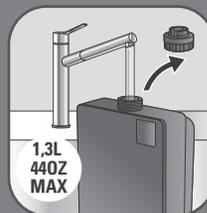
**EN** Remove the cap and fill in the water tank.
