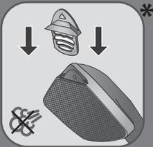
**EN** Insert the accessory inside the steam bonnet. Make sure the appliance is cold and not steaming during operation. Always use the steam bonnet with the MonParfum accessory inserted inside. You can use it with or without textile inside.
