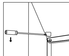
4. Move the core cover from left side to right side. And then lift the upper door and place it on a padded surface to prevent it from scratching.
