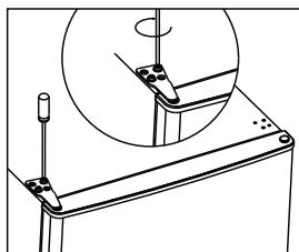
10. Clap in the hinge cover and hole cover on the top of unit.
