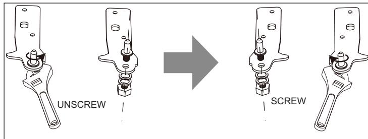
7. Install the hinge at left side and foot base at right side.
