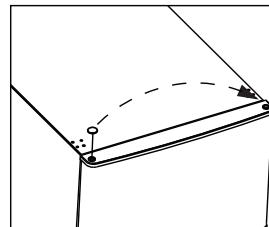
5. Lie down the rear of cabinet on a soft pad. And unscrew the bottom hinge and leveling foot.
