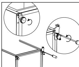
6. Unscrew and remove the bottom hinge pin, turn the bracket over and replace it.
